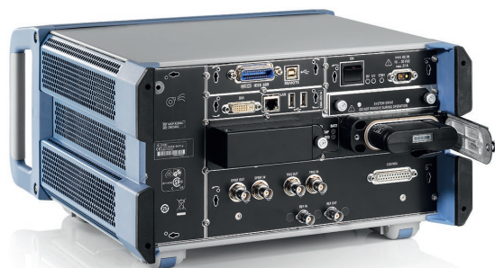
Fig. 4: Replaceable batteries enable interruption-free operation over long periods of time.
