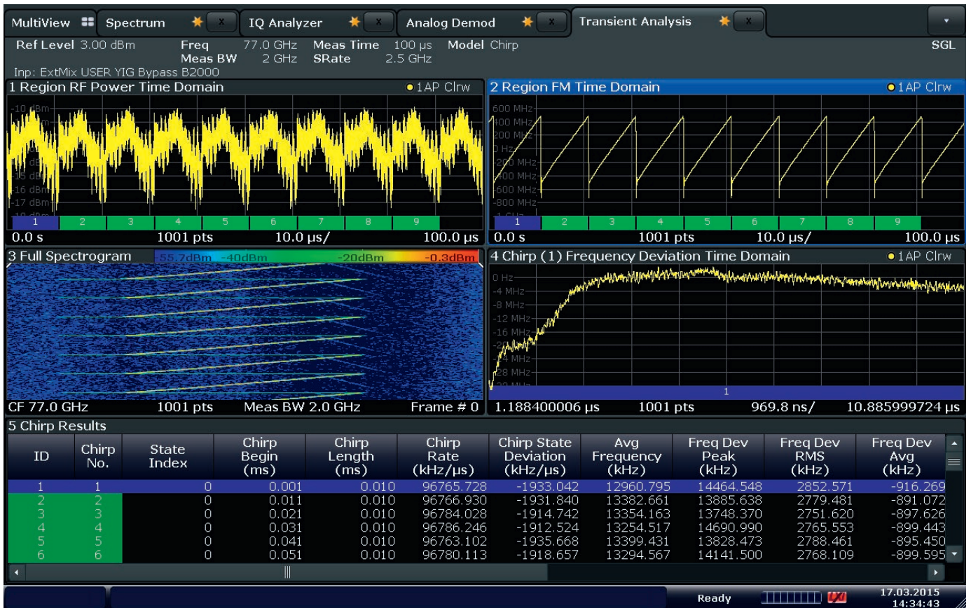
Fig. 5: Measurement of a 1 GHz FM chirp signal using the R&S®FSW-K60C option. Graphical depictions showing the frequency versus time or the power in the time domain. A table lists the most important measurement parameters.
