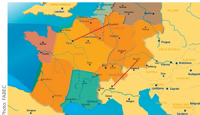
Fig. 1: Sample flight routes (red) with frequent ATC responsibility transfers in the small-scale airspace over Central Europe.
