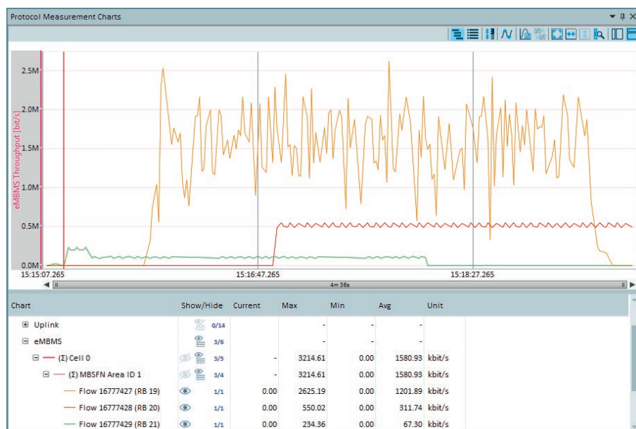
Fig. 6: For testing signaling scenarios and IP data streams, the R&S®CMWmars advanced extension graphically displays the eMBMS-specific measured values and data rates of each eMBMS flow / radio bearer separately for every MBSFN area.
